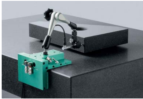
Squareness measurement with STRAIGHT-line 100
