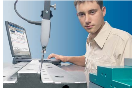
Straightness measurement on a guide way
